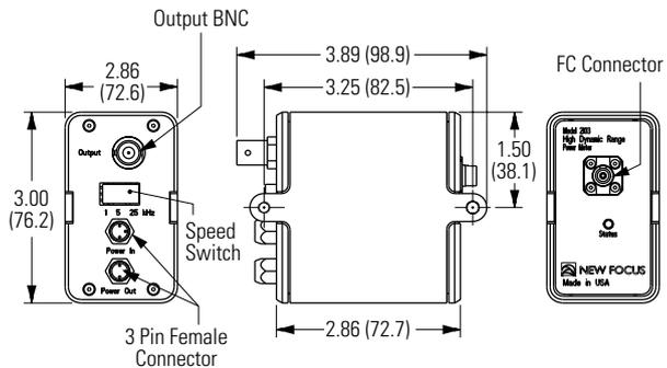
Unless otherwise noted, dimensions are in inches with metric dimensions in mm in parentheses.
