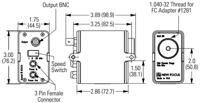
Unless otherwise noted, dimensions are in inches with metric dimensions in mm in parentheses.
